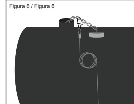
**Note:** If your fuel cap does not have a safety retention chain it may be necessary to modify the cap or tank lip to allow for the snap hook to be attached. Badly contaminated tanks may require the use of more than one cartridge to remove the water.
