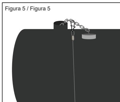
Slowly lower cartridge until it rests flat on the bottom of the tank. Check the cartridge in 6-12 hours to see if it has filled with water. If it is full replace with a new cartridge. If not, lower it back into the tank.
